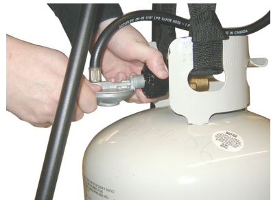
Figure 12 - Connecting Regulator to Propane/LP Gas Tank
